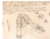
Cross-rolling process sketch of Max Mannesmann, pre 1885
